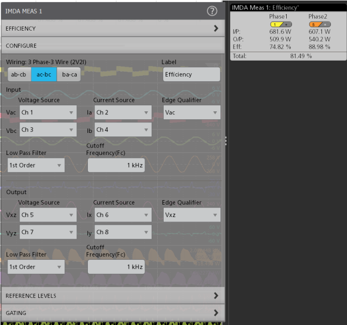
Configure wiring and filters to perform efficiency measurements
