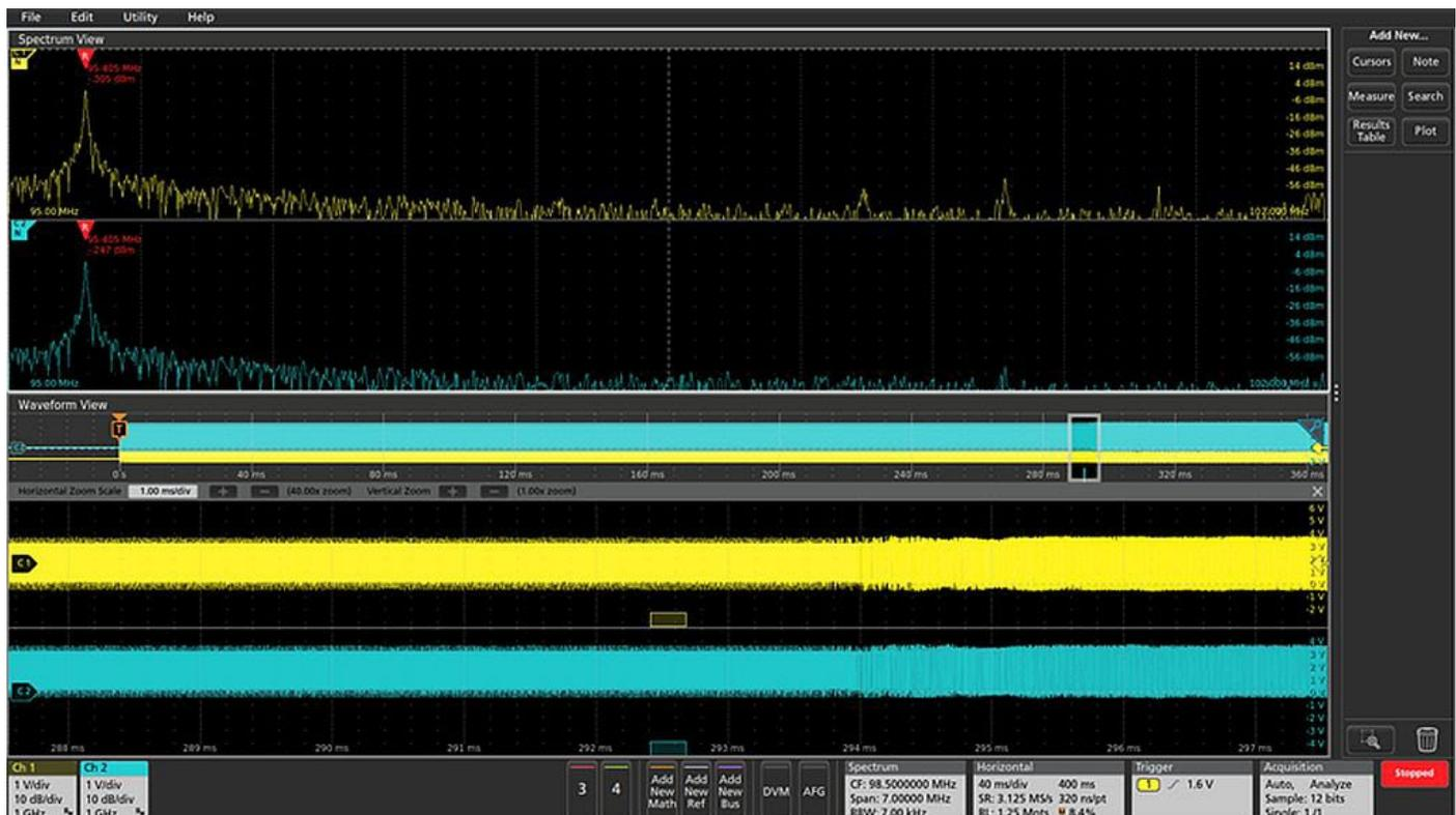
FIGURE 15. When debugging tasks demand it, multiple channels can be analyzed simultaneously. Here, two channels show the startup of a clock signal from two different points in a circuit.
