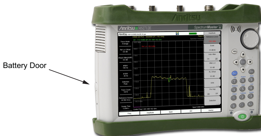
Figure 4-1. Battery Access Door Location
