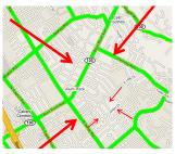
Direction Finding (DF) work is best done with a directional antenna, such as a Yagi, tuned to the band of interest. The DF process involves taking a series of directional readings, or bearings, of the suspect signal and recording those readings on a map. By
