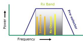
The unwanted, or interfering, signal does not need to be on the receive channel. If strong enough, it only needs to be within the radios' Rx duplexer or pre-selector frequencies.
