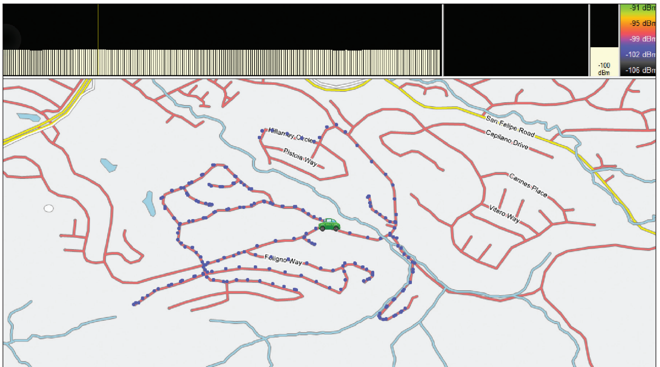
Figure 6. Multi-point measurement of a clean cable plant
