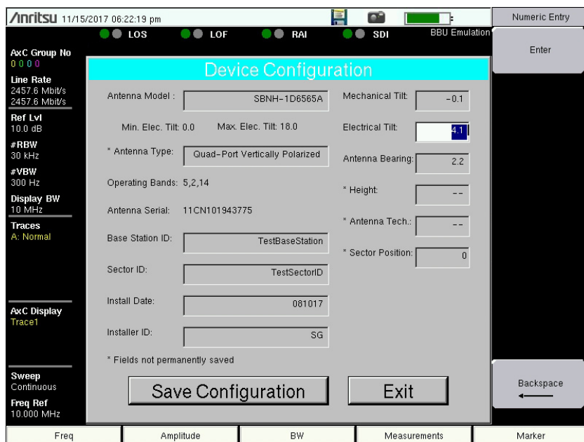
Figure 2-25. Electrical Tilt Entry
